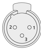
DMX-OUTPUT XLR mounting-sockets (rear view)
